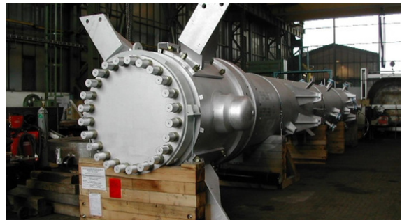
Waste heat boiler
